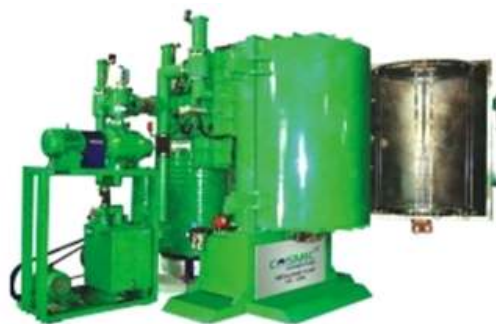
Vertical Coating Plant
